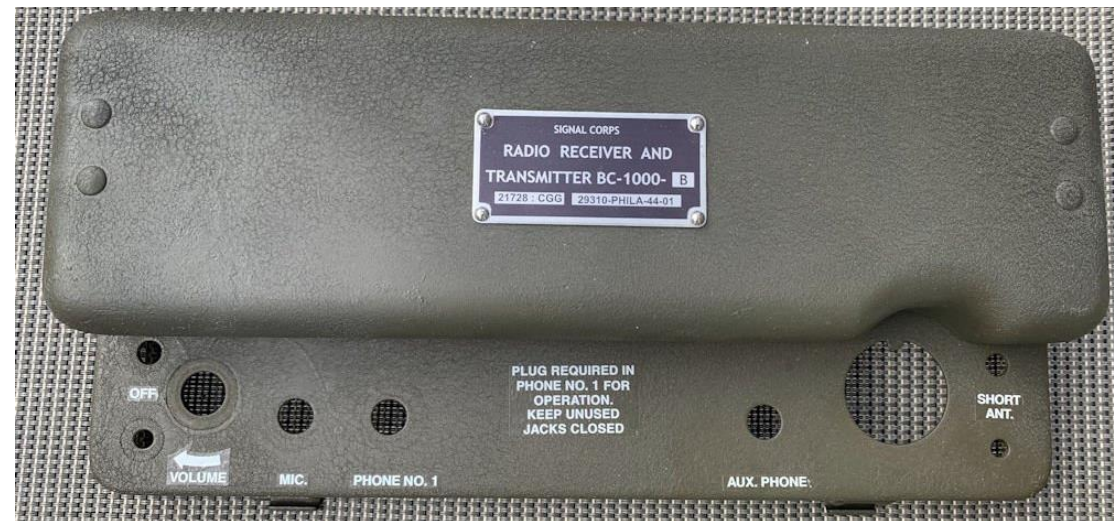
Installed using rivets on refurbished French BC-1000 top cover.
