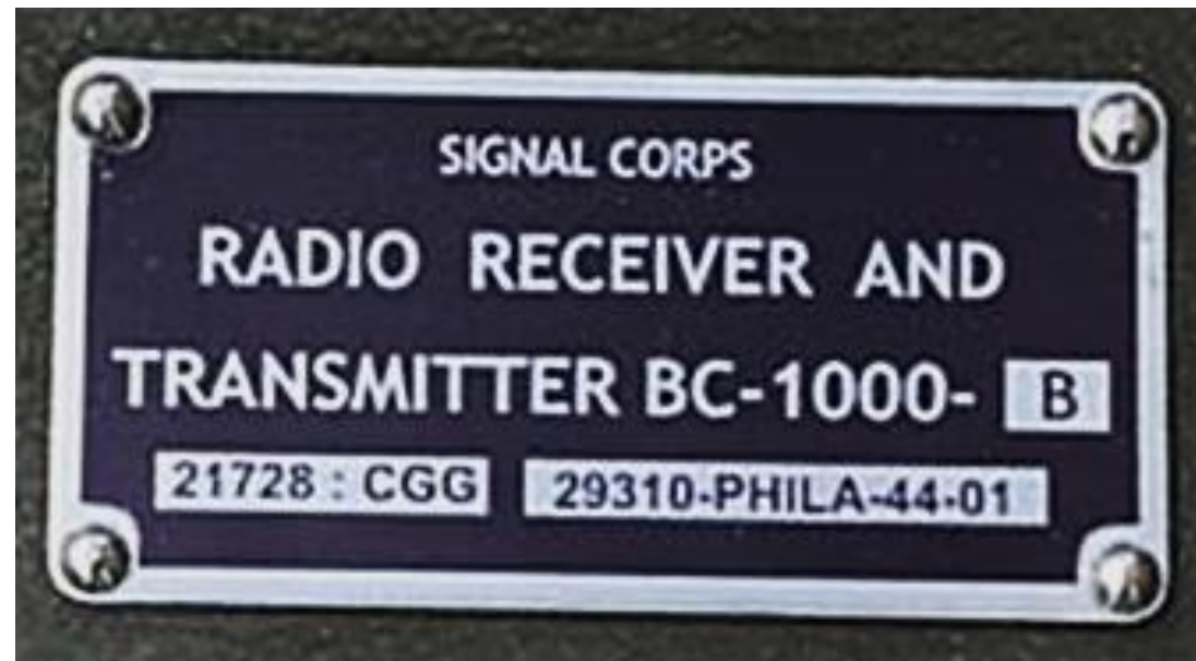
Installed using rivets on refurbished French BC-1000 top cover.
