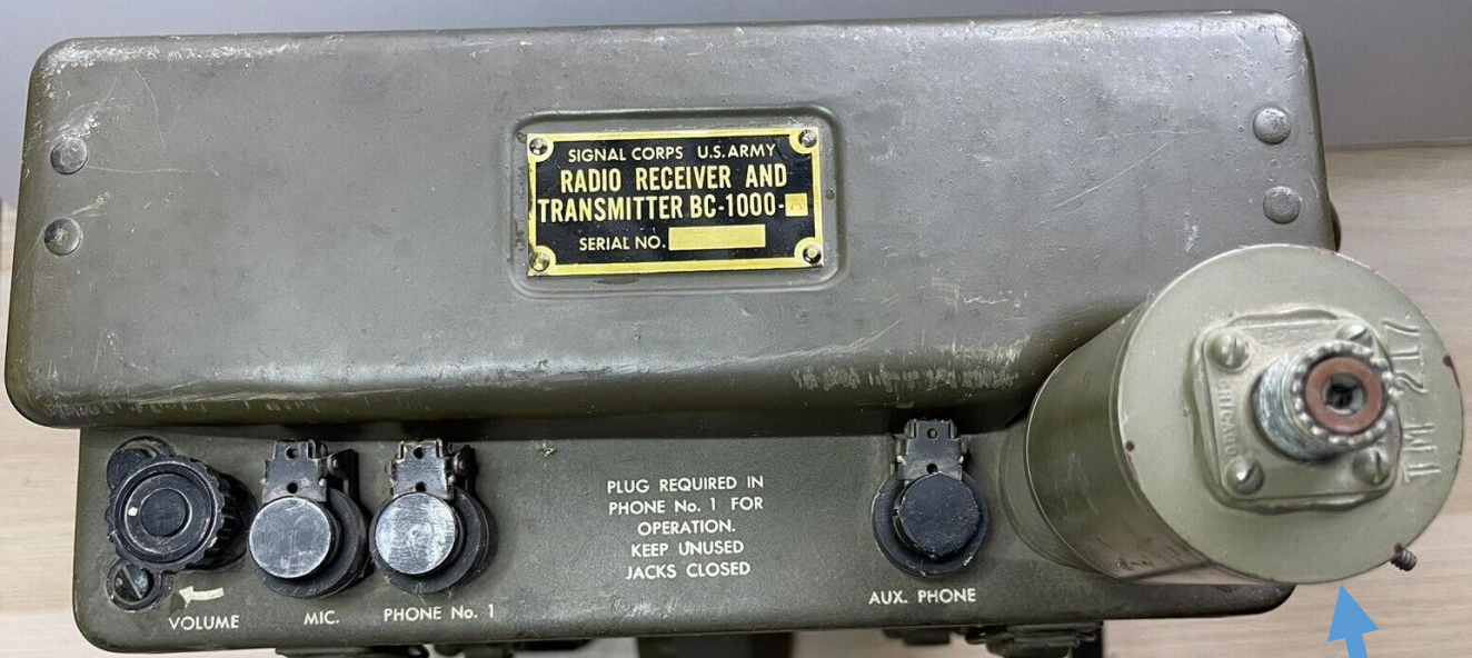
Observe the TM-217 Antenna Impedance Matching Unit required when using a coax cable to connect the BC-1000 to a vehicle antenna or to connect the SCR-300 to the RC-291 antenna system.
